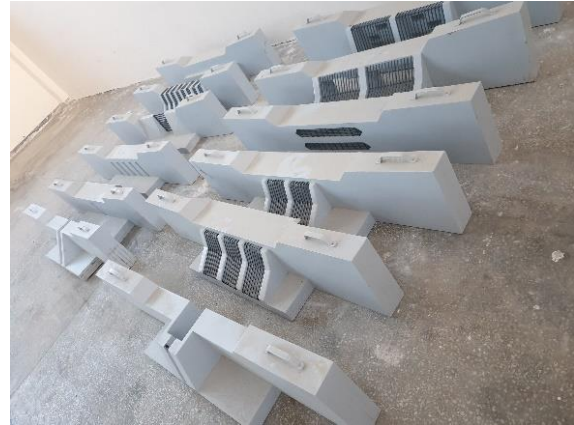
Fig. 29: Various types of boulder barriers have been tested and demonstrated in the model so far.
