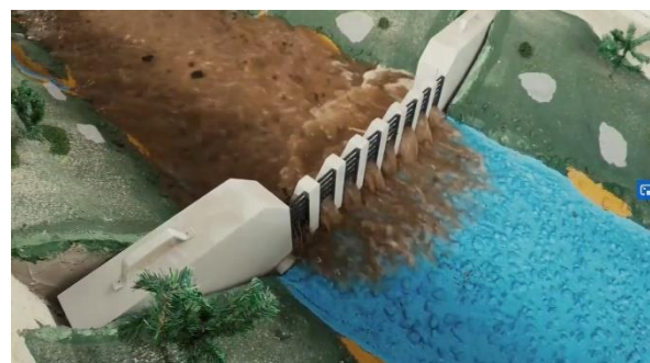
Fig. 33: Effect of another variant of the check dam on the model with driftwood
