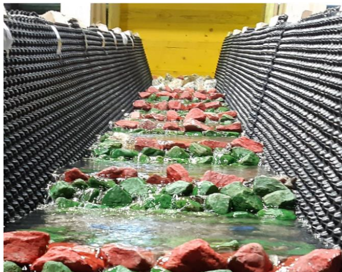
Fig. 35: Investigation of the stabilisation of the Maira riverbed at Promontogno by means of a stepped basin system
