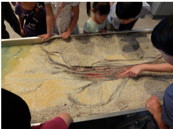
Fig. 78: Colour-coded sediments make transport phenomena visible according to grain size.
