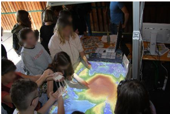
Fig. 95: In the Augmented Reality Sandbox, sand can be positioned in a landscape which is projected onto it as a topographical map. Here it is in use at the workshop in Heimschuh in 2019.
