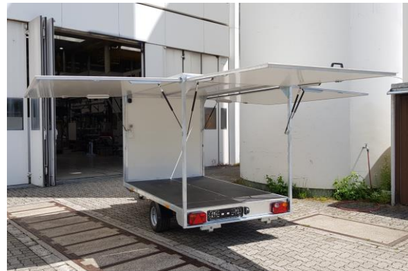
Fig. 101: The trailer can be opened on three sides and the low loading height allows children to access the model.
