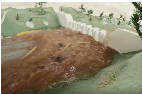
Fig. 32: Effect of a check dam in the model with driftwood
