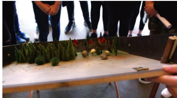
Fig. 57: Testing the protective measures with rocks by raising the flap.
