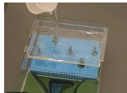
Fig. 71: Sponges simulate the retention effect of floodplains and forest areas.
