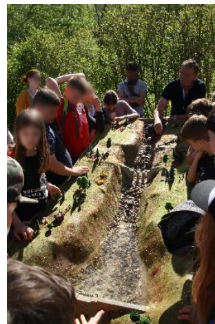
Fig. 25: The retention of debris and driftwood can be observed by the visitor.
