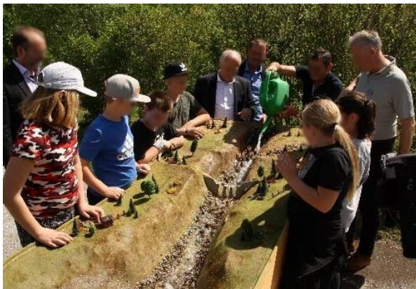
Fig. 22: The torrent model is filled with water. A bedload check dam is installed in the watercourse.
