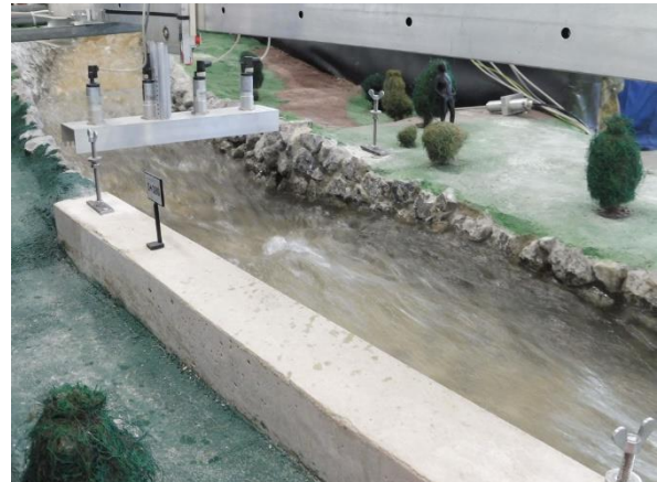
Fig. 51: In the case of HQ_{100} in the Wendelsteinbach, the village is protected by a wall of armourstone and a flood protection wall.
