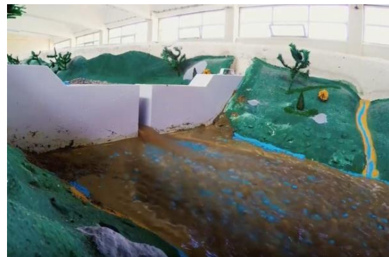
Fig. 31: Effect of a slotted dam in the model
