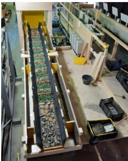
Fig. 34: Model for the river engineering measures on the Maira at Laboratorium3D
