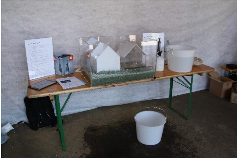
Fig. 60: The uplift model for houses of the Department of Water Management of the Upper Austria Regional Government, here at the workshop in Heimschuh in 2019.
