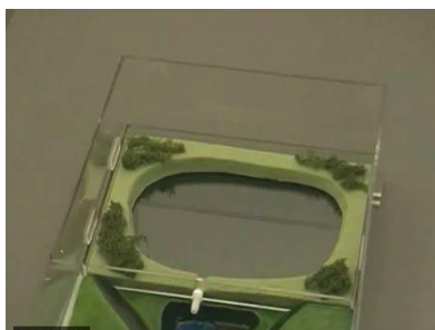
Fig. 69: A retention basin is created in the inlet to hold water.
