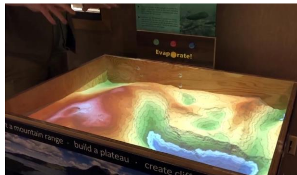
Fig. 96: After creating the topography, rain can be simulated, which then flows as it would in the real landscape.
