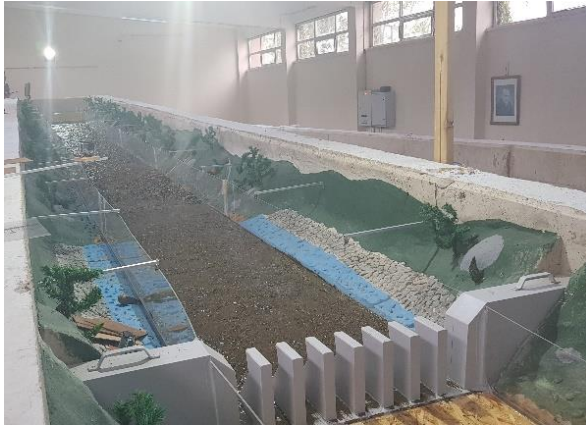
Fig. 28: Check dam model in the Turkish Flood Museum after construction
