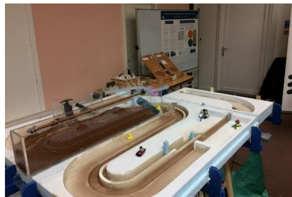
Fig. 73: Photo of the Wetropolis model with view of the marsh reservoir
