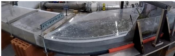
Fig. 52: The covered channel of the Larchbach becomes blocked with heavy influxes of alluvial wood.
