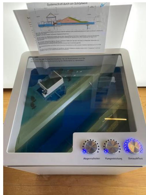
Fig. 59: Model of the pumping station during a flood situation in the Danube
