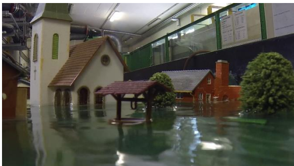
Fig. 38: Flooding in the settlement area is clearly depicted.
