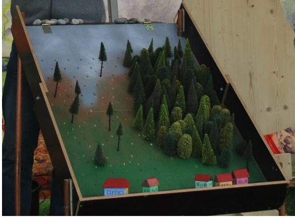
Fig. 54: The rockfall model with the movable forest area on the left and the protective forest on the right. The village affected lies below. The rocks can be seen at the top.
