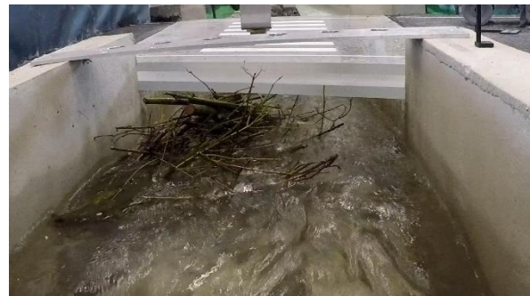
Fig. 53: Accumulations of driftwood can also lead to blockages at the bridges in the village, which can block the upper course.
