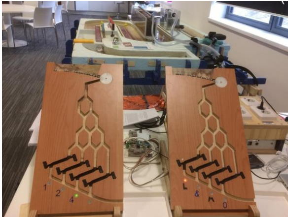
Fig. 74: Galton boards for controlling the duration, intensity and location of precipitation.
