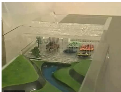
Fig. 66: Precipitation falling on a sealed car park area is simulated by adding water.
