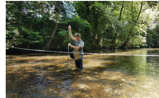
Teledyne RDI's StreamPro ADCP can simply be pulled across the stream as you walk across a bridge, or attached to a tagline to collect real-time data.
