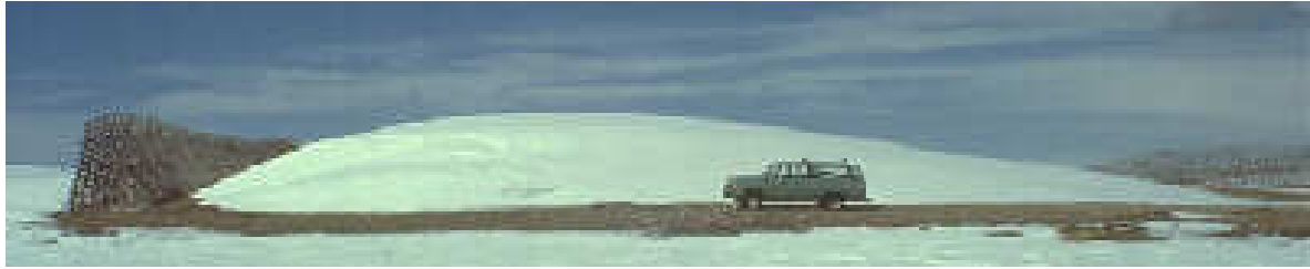
Figure 25 : In this photo, the drift downwind of a 12.4-ft Wyoming snow fence is near equilibrium ( Tabler 1986 ). Wind is from the left, from www.wrds.uwyo.edu/
